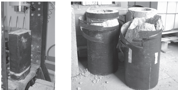
Figure 4 – Failure of FRP- wrapped specimens
